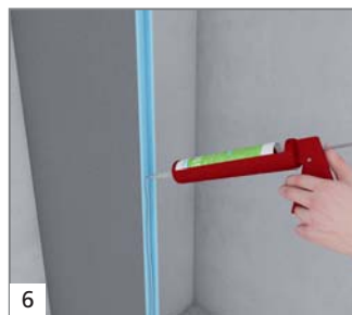
6 Before installing the tongue, an evenly applied layer of wedi 610 adhesive sealant is applied in the groove.
